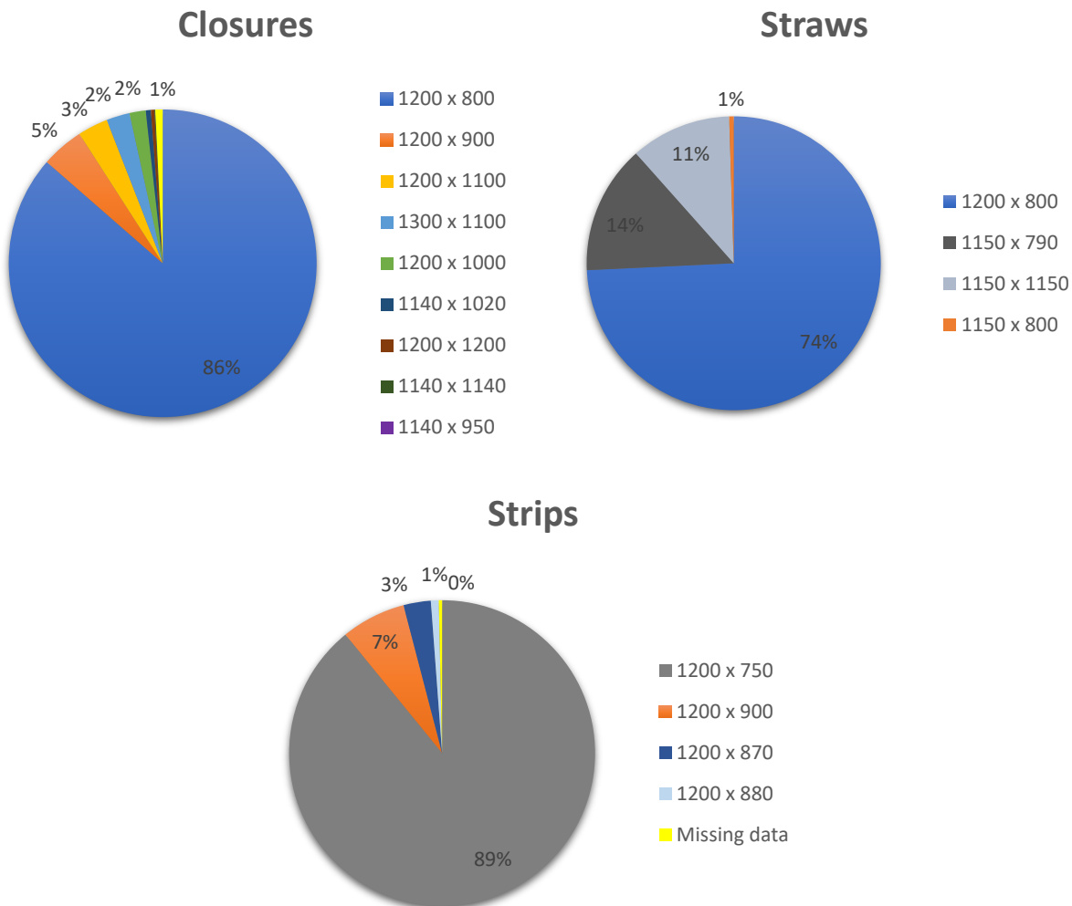
Figure 5: Charts over the distribution of pallet sizes used for shipments for each product area. The data is based on the 374 940 pallets shipped by AddMat in 2018 (Shipments originating in Europe, Films excluded). The pallet sizes are in order according to the number of uses. Some products did not have any information on pallet sizes used, hence the “Missing data”.
